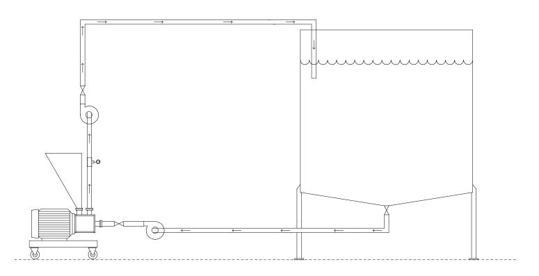
Example #3 describes the Inline SLIM System being used with a large (1000+ gallon) recirculation vessel. The Inline SLIM unit is located on ground level and is not close to the outlet of the tank, therefore, a centrifugal pump is used to feed the inlet side. Since the discharge tubing is long, a centrifugal pump is used to minimize the back pressure on the discharge side.
