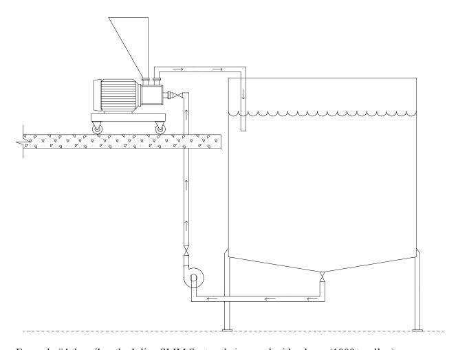
Example #4 describes the Inline SLIM System being used with a large (1000+ gallon) recirculation vessel. The Inline SLIM unit is located on an elevated mezzanine or upper level floor. The inlet of the Inline SLIM is not close to the outlet of the tank, therefore, a centrifugal pump is used to feed the inlet side. Since the discharge tubing is short, the discharge side does not require a pump.
