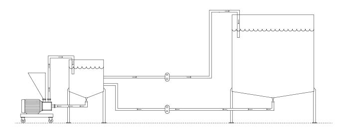
Example #5 describes the Inline SLIM System being used with a large, remote storage tank. A small (50-500 gallon) recirculation buffer vessel is mounted near the Inline SLIM unit. The Inline SLIM unit is located on ground level and is as close to the outlet of the recirculation vessel tank as possible. Discharge tubing length is kept to the minimum possible length.
